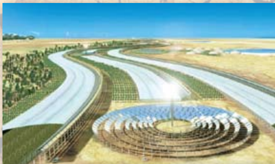
Charlie Paton is the author of the Sahara Forest Project, which is a scheme to provide fresh water, food and renewable energy in hot, arid regions as well as re-vegetating areas of desert. The scheme combines two established technologies – the Seawater Greenhouse and Concentrated Solar Power – to achieve highly efficient synergies.
